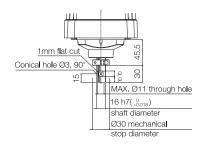
Detail view from "A" (Calibration point position of joints #3 and #4)
